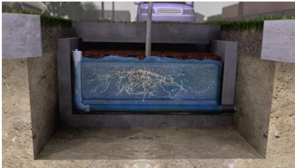
Figure 46: Cross-section of a Filtterra System
