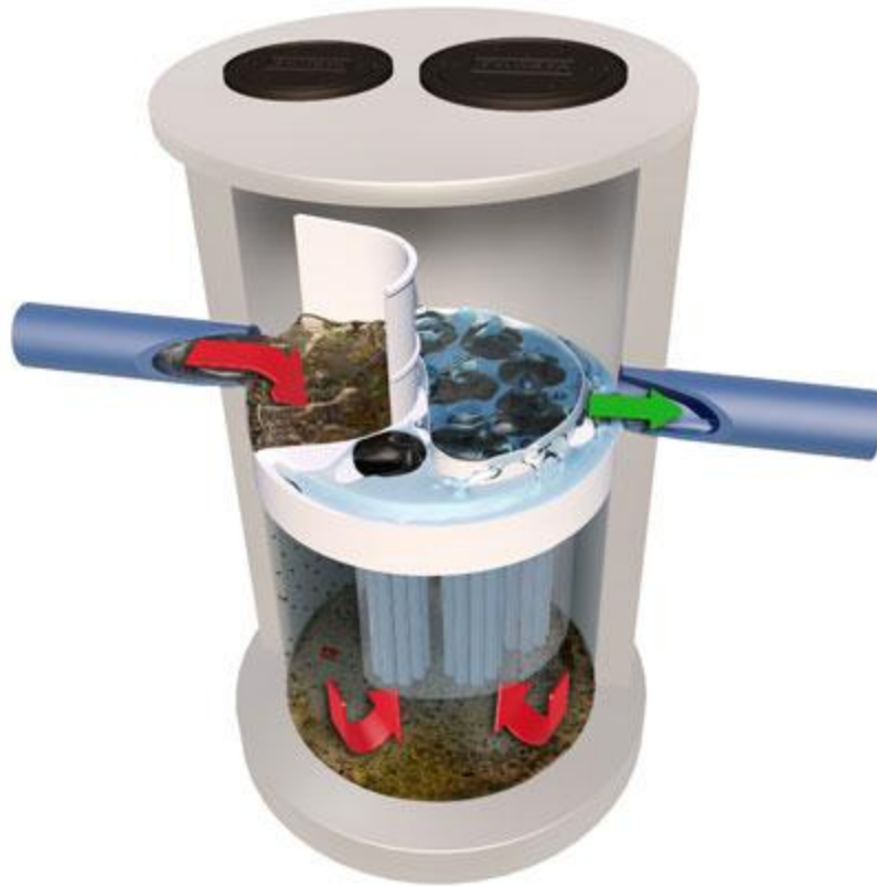
Figure 48: Diagram of the Jellyfish Filter
