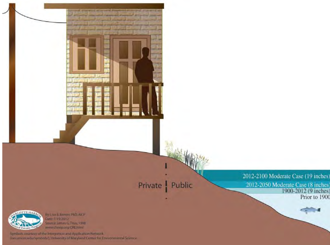
Figure 184: Rolling easement step 3 Year 2100. Moderate case 20 inches sea level rise. Marsh moves inland. Former marsh becomes inundated. Source: CHNEP 2009 Based on Titus 2000.
