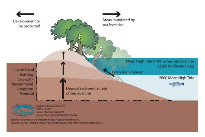
Figure 22: A method of gradual filling of areas in front of shoreline protection.
